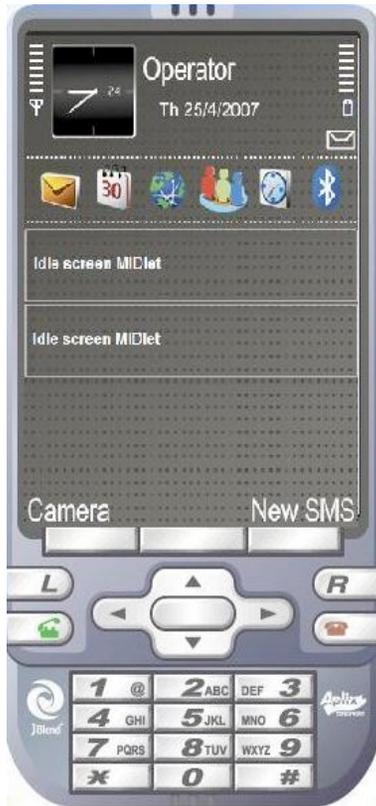
An **Idle Screen MIDlet** is a normal MIDlet that has an additional UI component (**IdleItem**), which is rendered on the idle screen.
